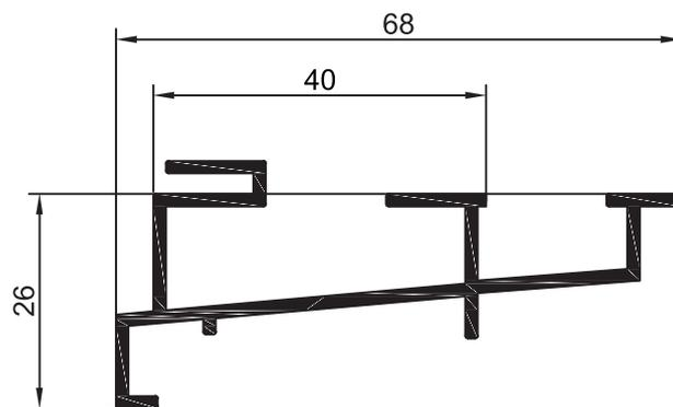
**AN.83** *Soleira Condensação*
